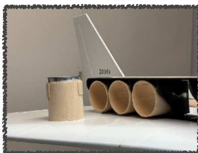
Glued wood sections around a wax paper covered can and primed and painted six exhaust ducts. Paint dried and held the shape.
